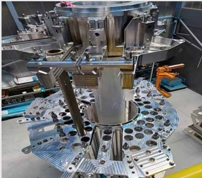
RJH: FACTORY ASSEMBLY OF THE RJH REFLECTOR
