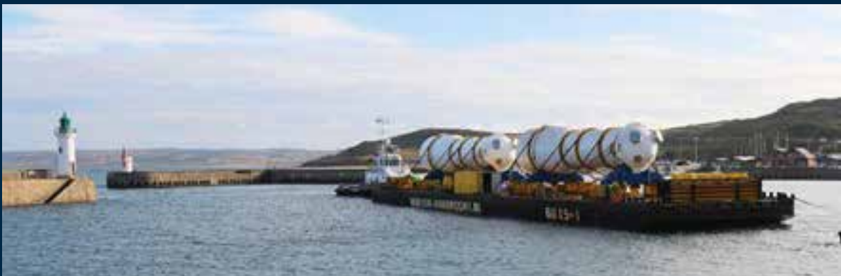
FLAMANVILLE REPLACEMENT STEAM GENERATOR ON A BARGE
