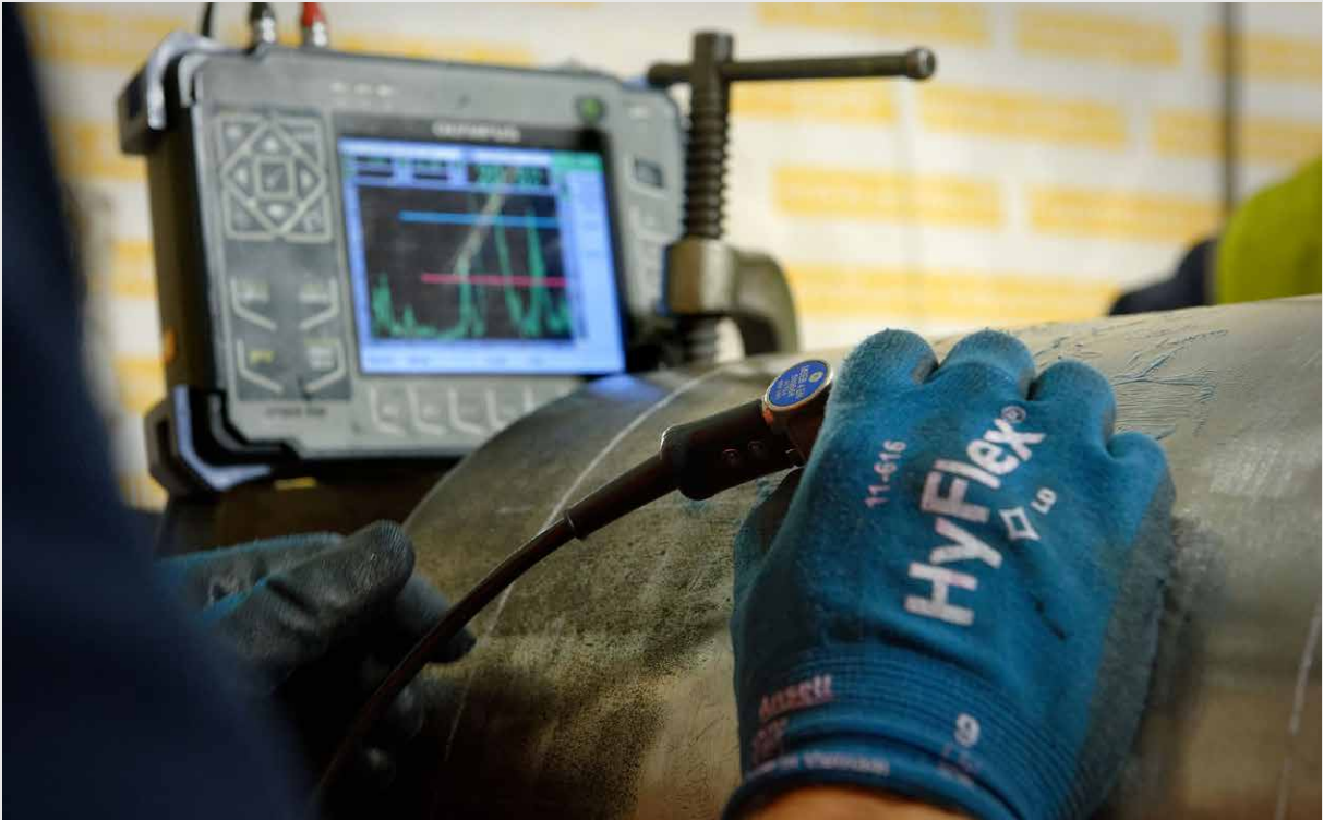
ULTRASONIC EXAMINATION OF WELDS
